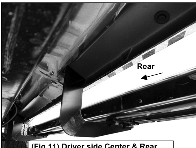
(Fig 11) Driver side Center & Rear Brackets attached to Running Board
